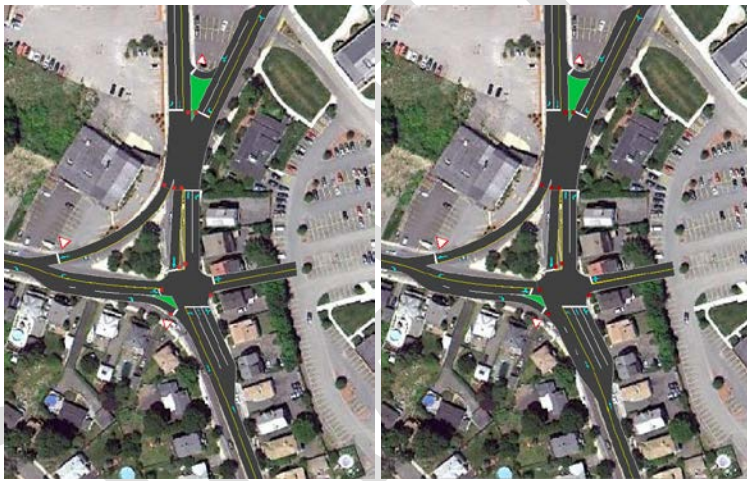
Figure 11. New northern driveway Figure 12. New northern driveway with added southbound departure lane
