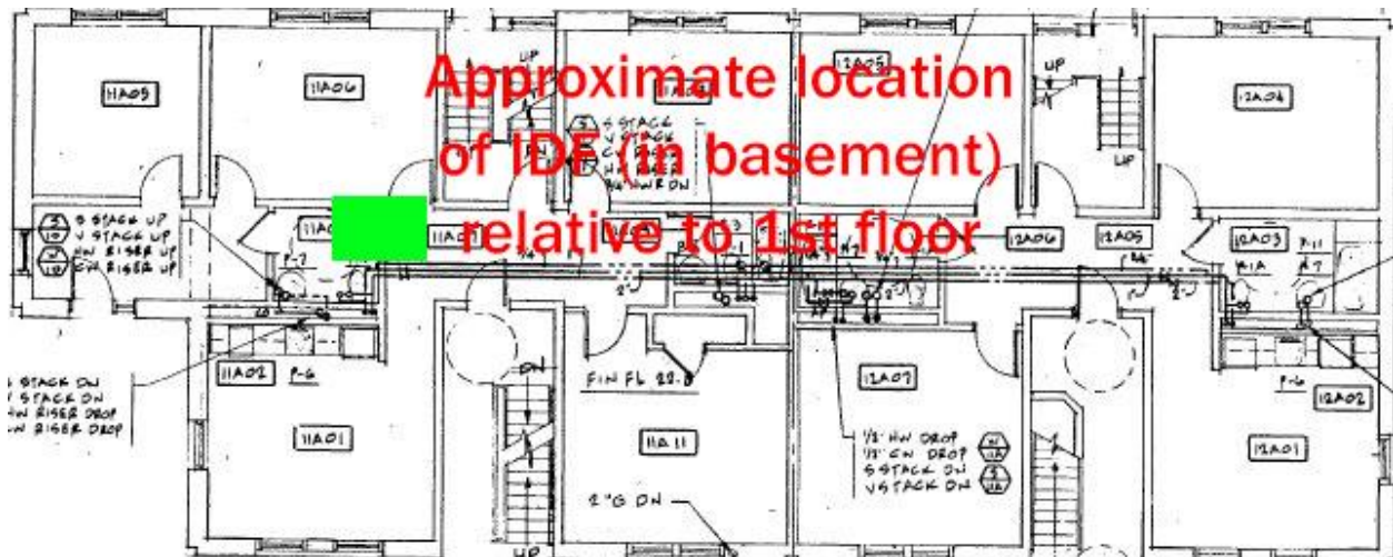
Bates E_1st Floor_FloorPlan_and_IDF-location
